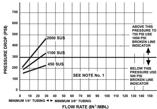
Table 2. Broken Line Indicator-Maximum Line Lengths Permitted in Grease Systems
